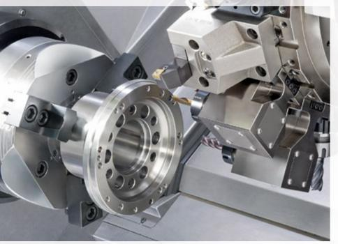
The B750 and B1250 machines are equipped with the new turret with a direct drive built-in motor and feature a sturdy cast-iron machine bed. Particularly suitable for the machining of flanges and shafts with high chip removal, the B1250 features a long bed with a longitudinal stroke of 1310 mm, large bar capacity and a sturdy CNC automatic tailstock with a 115 mm hydraulic quill. The B1250 can accept the travelling steady-rest.
