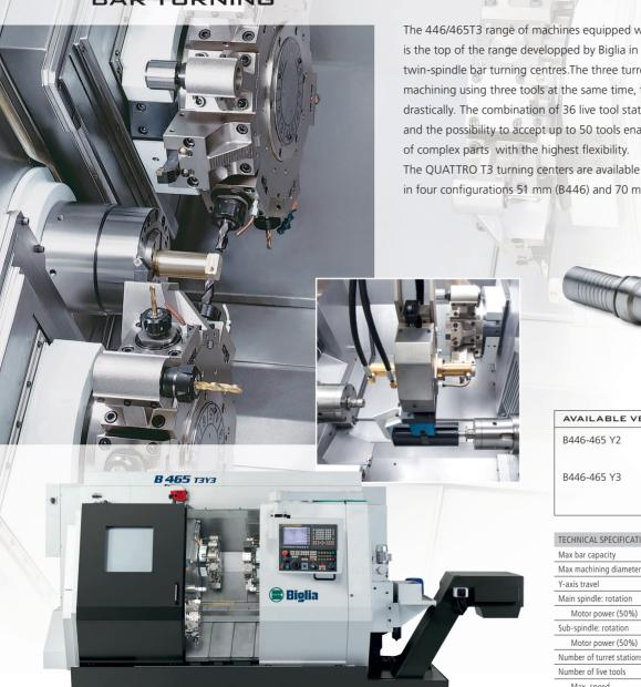
The 446/465T3 range of machines equipped with three turrets and thirteen axes is the top of the range developped by Biglia in the field of high-performance twin-spindle bar turning centres. The three turrets can perform simultaneous machining using three tools at the same time, thus reducing cycle time drastically. The combination of 36 live tool stations, 3 Y-axes, 2 C-axes and the possibility to accept up to 50 tools enables the complete machining of complex parts with the highest flexibility.
